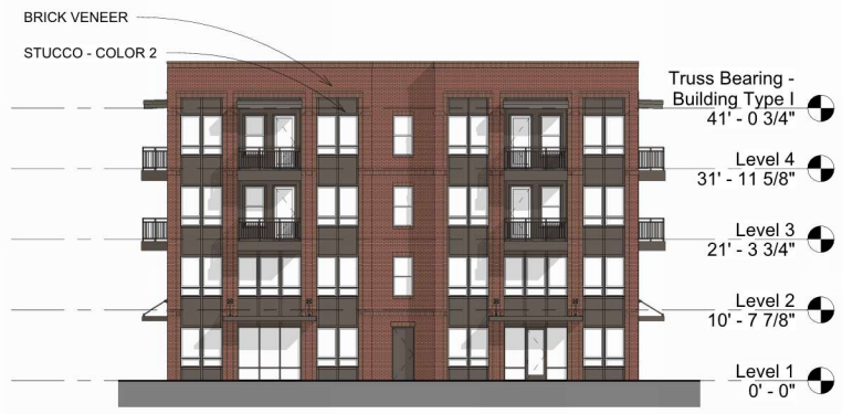
4 Building 1 - Northeast Overall Elevation 1/16" = 1'-0"
