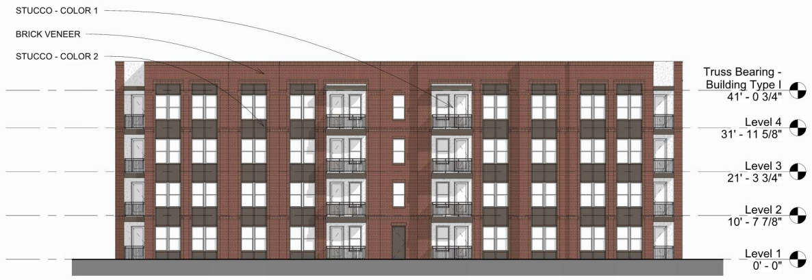
3 Building 1 - West Overall Elevation 1/16" = 1'-0"
