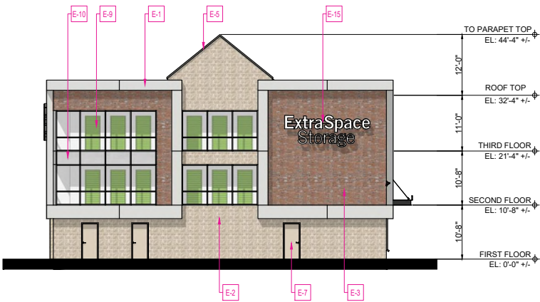
NORTH ELEVATION - 80.3% MASONRY COVERAGE
