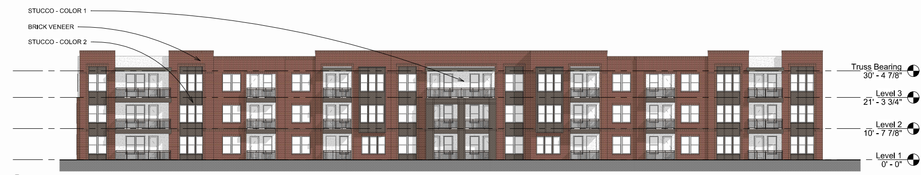
2 Building 3 - West Overall Elevation 1/16" = 1'-0"
