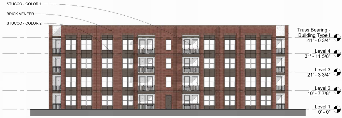
3 Building 1 - West Overall Elevation 1/16" = 1'-0"
