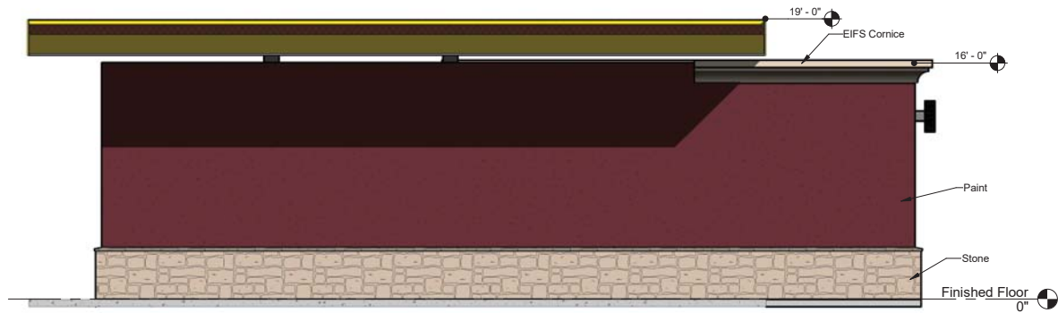
③ Service Bay Left Elevation 3/16" = 1'-0"
