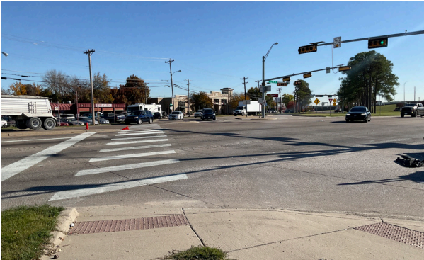
The roadway geometry of Mill St results in long crossing distances for pedestrians.
