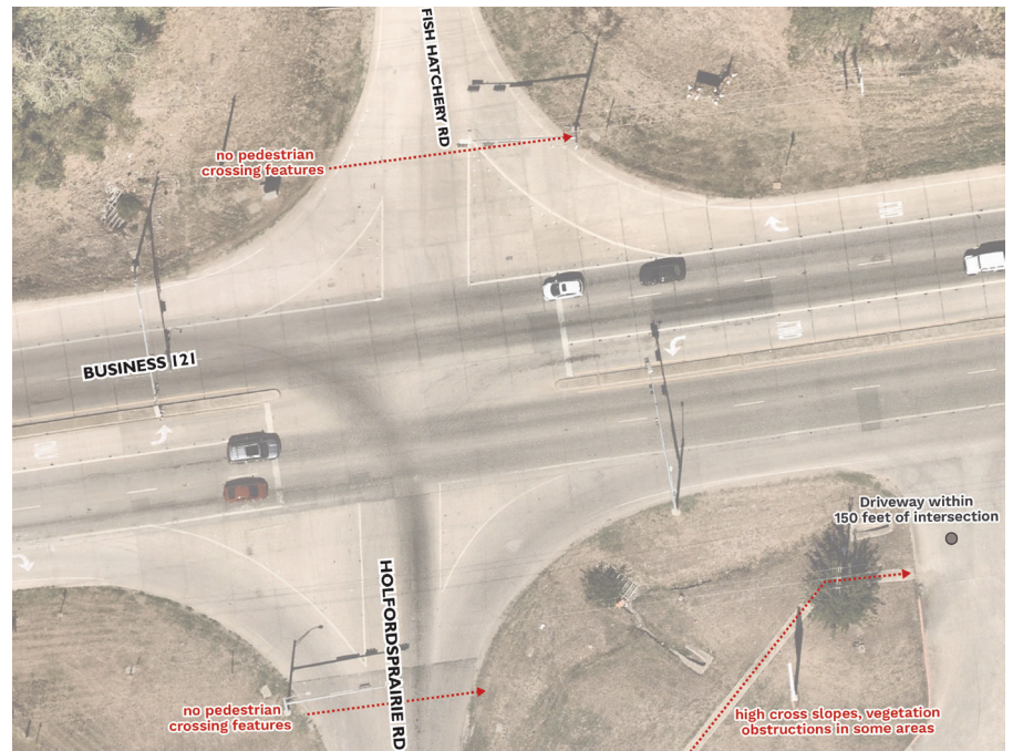
Fig.78: Fish Hatchery/Holfords Prairie Intersection Key Issues
