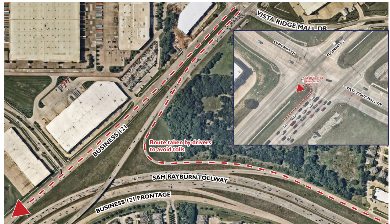
Fig.22: Dedicated U-Turn Lane at Vista Ridge Mall/Edmonds Lane
