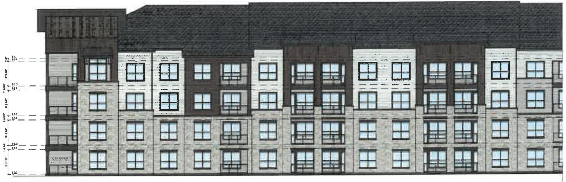
1a BUILDING C ELEVATION - SOUTH SCALE: 1/4"=1'-0"
