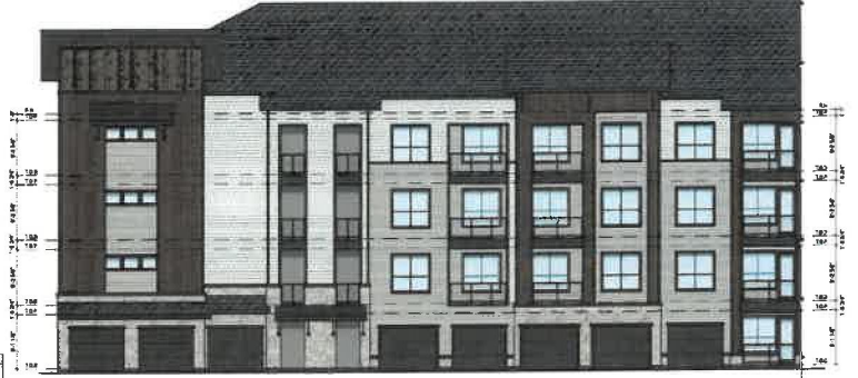
4 BUILDING C ELEVATION - WEST SCALE: 1/8"=1'-0"
