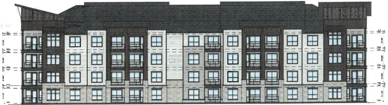
1 BUILDING B ELEVATION - EAST SCALE: 1/8" = 1'-0"
