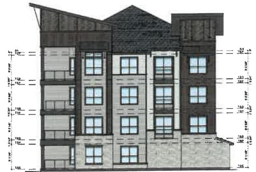
2 BUILDING B ELEVATION - NORTH SCALE: 1/8" = 1'-0"
