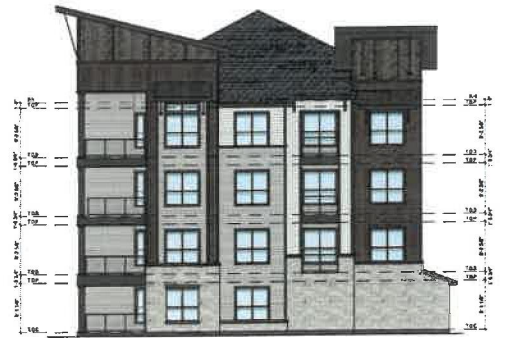
2 BUILDING B ELEVATION - NORTH SCALE: 1/8"=1'-0"
