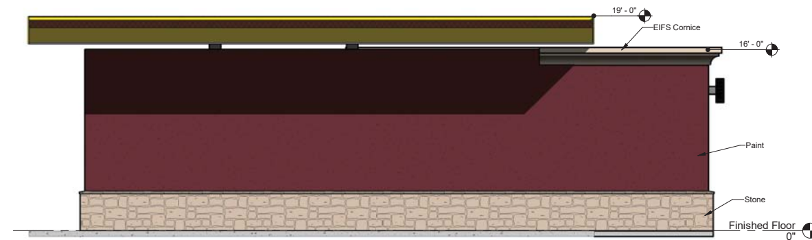
③ Service Bay Left Elevation 3/16" = 1'-0"
