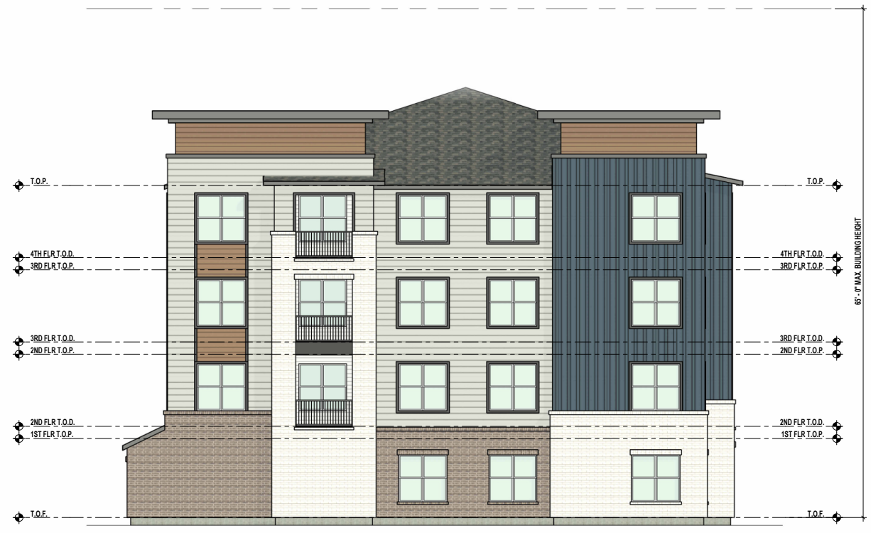
7 BUILDING A ELEVATION 1/8" = 1'-0"
