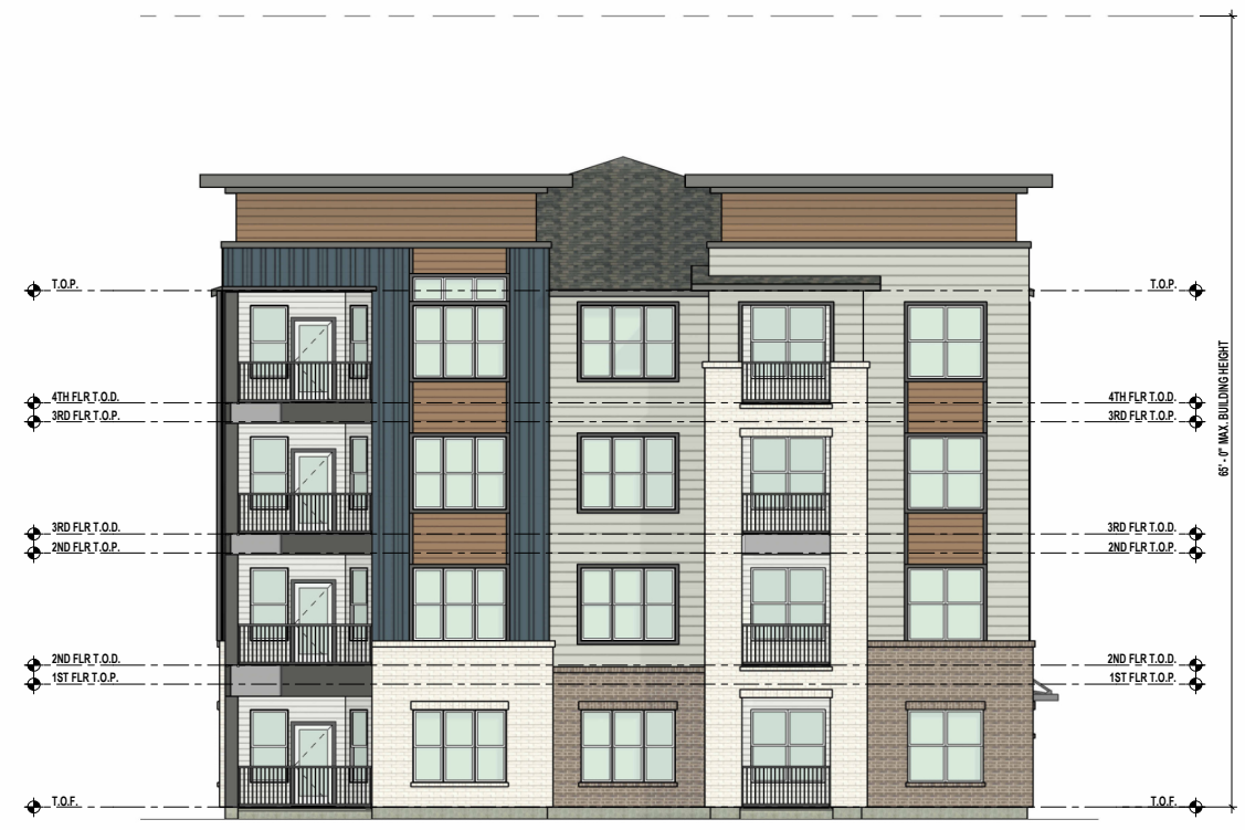
3 BUILDING A ELEVATION 1/8" = 1'-0"
